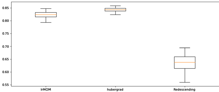
Fig. 14 Boxplot of the accuracy obtained on 50 training/test run (2000 training sample, 2% corruption) of each algorithms on a 200-dimensional toy dataset
