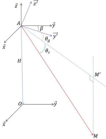
Fig. 1: A reflecting point on the ground represented by its angular coordinates with respect to the center of the radar antenna
