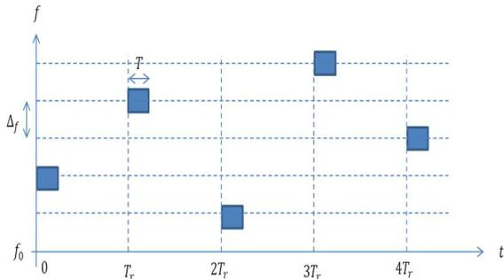
Fig. 7: Time-frequency graph of a step frequency waveform
